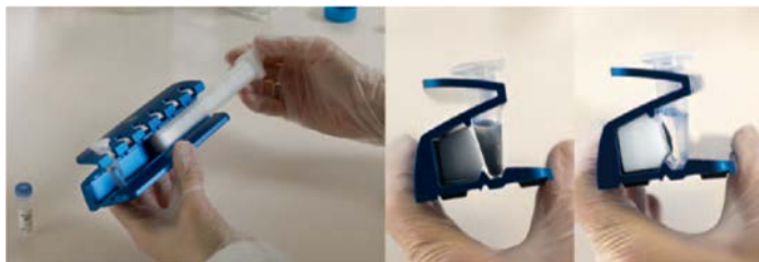
Fig 3.27. The high density of Mag Sepharose beads allows rapid capture by MagRack 6 magnetic device.
