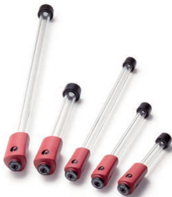
Fig 3.3. Empty Tricorn columns for packing. Once packed, these columns can be used for purification using either a pump or chromatography system.
