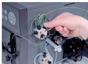
Fig A4.2. Typical procedures using ÄKTApurifier plus. (A) Prepare the buffers. (B) Connect the column. (C) Prepare the fraction collector. (D) Load the sample.
