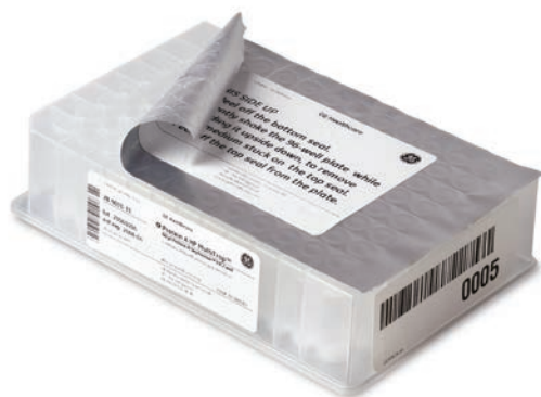
Fig 3.15. Protein A HP MultiTrap 96-well plates are used for rapid, parallel screening and small-scale purification of monoclonal and polyclonal antibodies.
